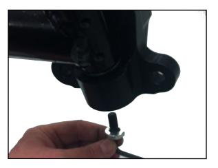
LINE THESE INDENTS UP WITH THE SET SCREW HOLES IN THE AXLE
