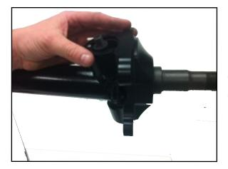
STEP 5 Drop the kingpin into place and push it down through the steel cup washer and into the lower bearing until it bottoms out. Take the bottom kingpin bolt and the aluminum washer and screw it into the king pin, just snug it.
