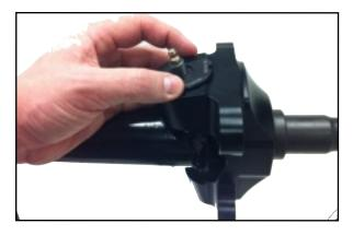
Take your camber pill of choice and grease the inside of the bushing lightly. Note, when putting the pill in the POS stands for the positive side of the pill....What this means is if POS faces the tire it is giving it more positive camber.
